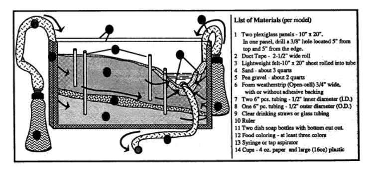
Station/student 2 - collect plastic soap bottles, tubing (1/2" I.D. and 1/2" O.D.), foam strips, and syringe or other aspirator. Force foam up about one inch into each of the large (1/2" I.D.) pieces of tubing for use in step 5.
