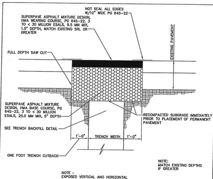
NOTE: EXPOSED VERTICAL AND HORIZONTAL SURFACES SHALL BE PREPARED AS STATED IN PENNDOT PUB 408, SECT. 413.3(g).
